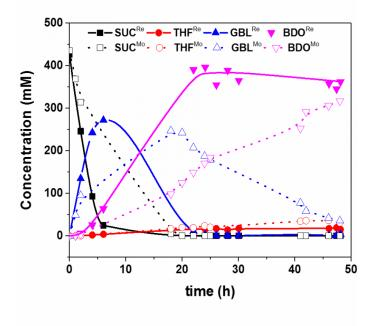
FIGURE 1 Hydrogenation of SUC (5%, 160 degree C, 150 bar H2) 2%Pd (tol) /(5%ReOx-TiO2 NHSG) or 2%Pd (tol) /(4%MoOx-TiO2 NHSG)
