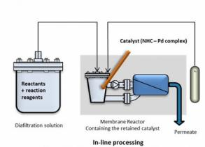
((semi)-Continuous conversion-separation process)
